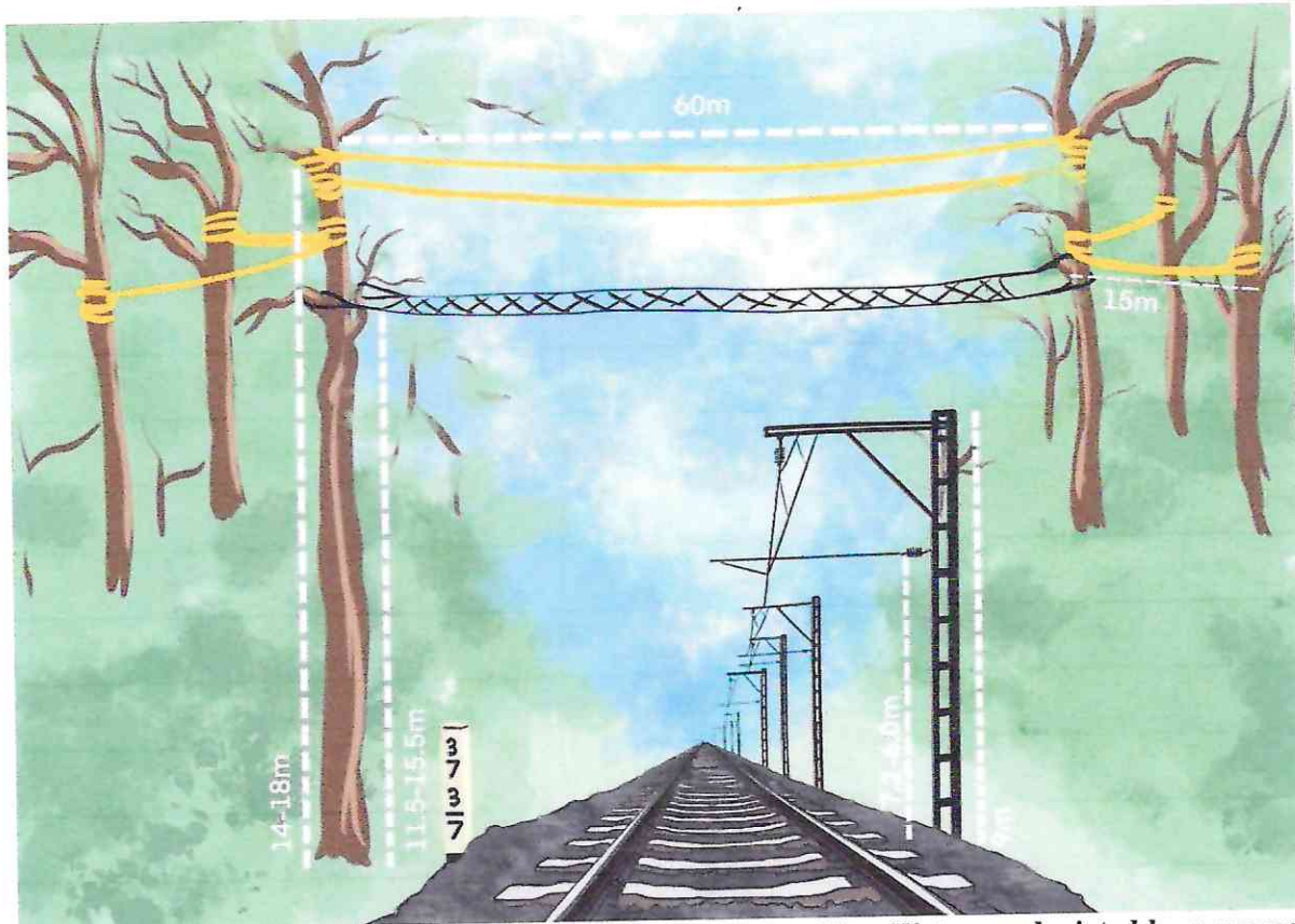
Figure 17: An illustrative example of an artificial canopy bridge (distances depicted here are not to scale) design at HGS incorporating concerns shared by Railway authorities factoring in the near-future electrification prospects of the railway line (illustration by Vabesh Tripura)
